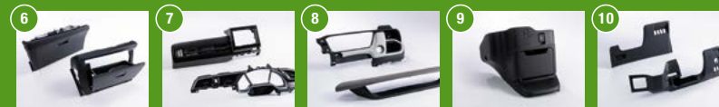
6 Glove compartment 7 Center cluster & ventilator 8 Meter visor 9 Center lower cover 10 Instrument panel lower cover (driver side)
